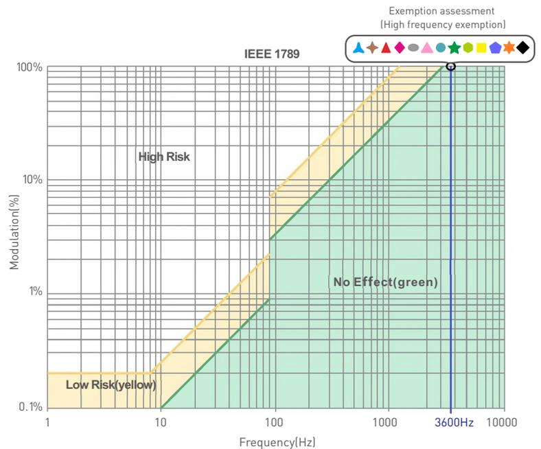
Marks in the right chart are tested results of different current levels. The output frequency is 0Hz in 100% brightness and its corresponding modulation is 0%, which could not be shown in the right chart.
