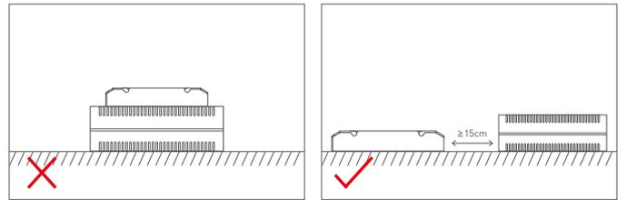
Please not place the products on LED drivers. The distance between the product and the driver should be  $\geq 15\text{cm}$  so as not to affect heat dissipation and shorten the lifespan of the products.
